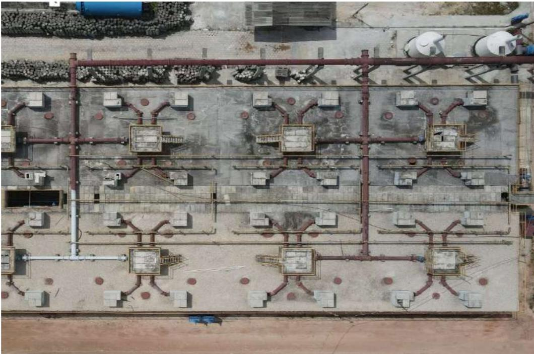
*Figura 286. BEL017-ETE Una, reator UASB retangular.*
